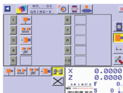
Main screen of the internal grinding (with internal grinding attachment option)
